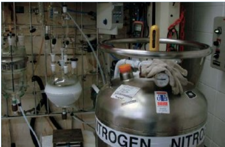
Albemarle uses liquid nitrogen cooling on this 10-litre, low temperature laboratory apparatus
